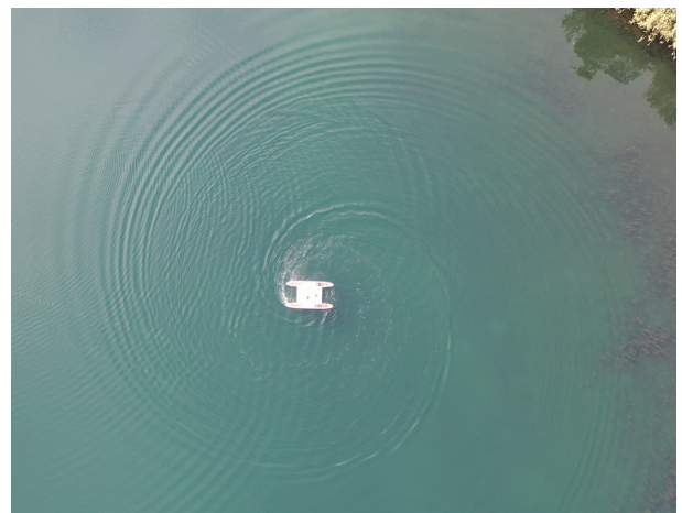
(b) Top-view of the spiral executed by the vessel. Note the waves hinting the vessel's trajectory.
