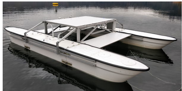
Fig. 1: Nukhada USV, TII’s new USV for autonomous survey, inspection, and support to underwater robotic operations.
