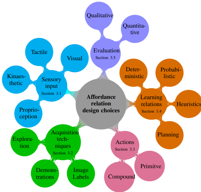
Figure 3: Design choices to build affordance relations as considered in this survey. Starting at the top-left branch and counter-clockwise, we outline the options found in the literature for collecting data in terms of sensory input (blue) and acquisition techniques (green). We also look at the type of actions used to build an affordance relation and perform a task (rose). Once the type of affordance elements have been chosen, we outline the different learning methods employed to relate those elements (orange). Finally, we review the different metrics for evaluation of the affordance task (purple).
