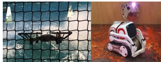
Figure 3: Left: One of the drones (approx 12 cm in diameter), in its netted enclosure. Right: A Cozmo (foreground) with a circular Limpet [39] sensor attached to the wall behind.
